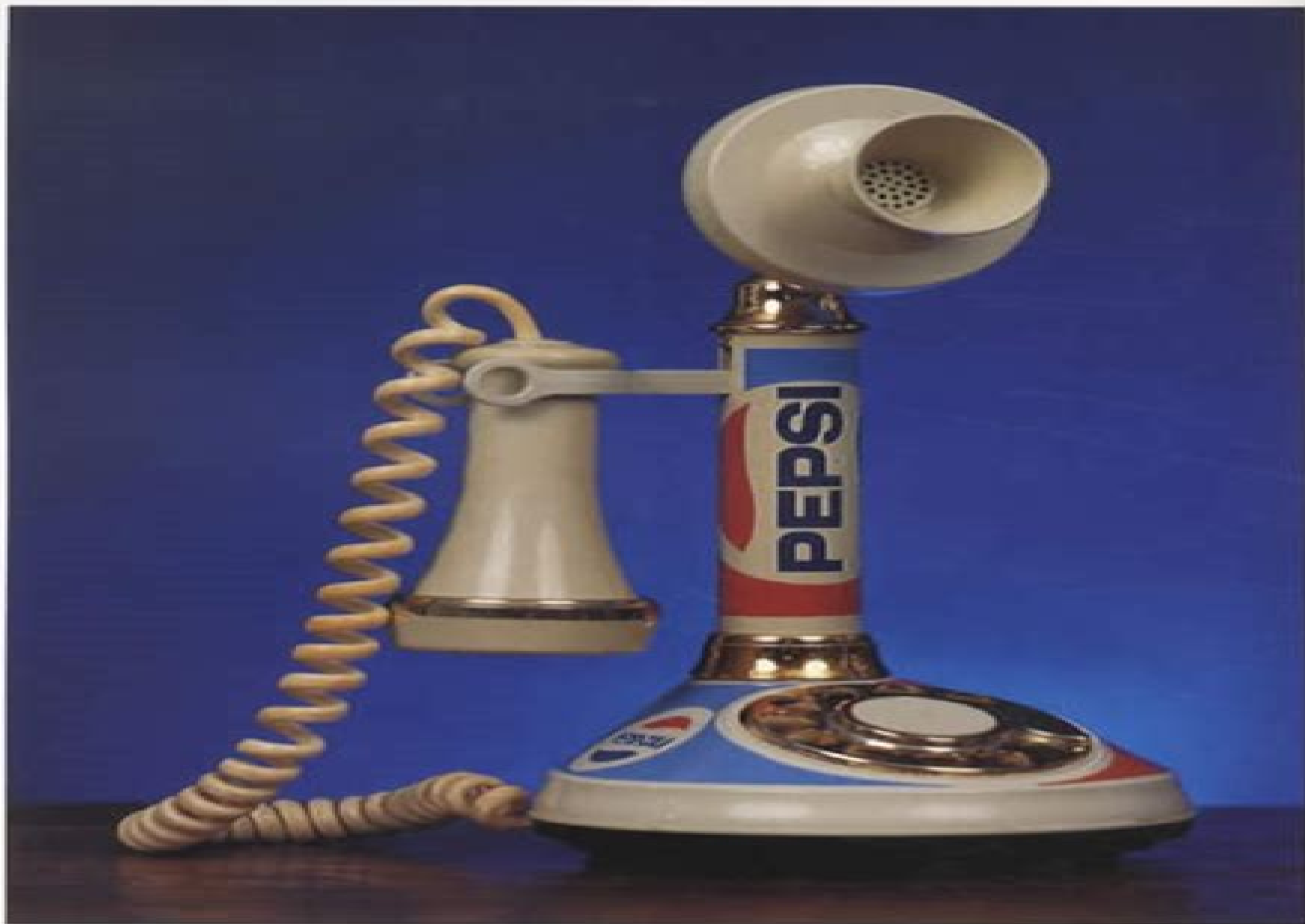
The Pepsi Candlestick Telephone was made in the U.S.A. by American Telecommunications Corp., El Monte, California, 1974. 12" H x 5.75" diameter. Pulse dialing. Transmitter mouthpiece. Receiver handset. On/off hook switch on side of stick. Desk set. $95-140.
