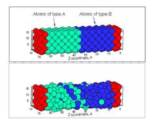
Inhomogeneous materials can become homogeneous by diffusion. For an active diffusion to occur, the temperature should be high enough to overcome energy barriers to atomic motion.
