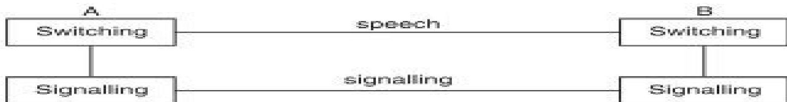
(a) Common-channel signalling between A and B on an associated basis
