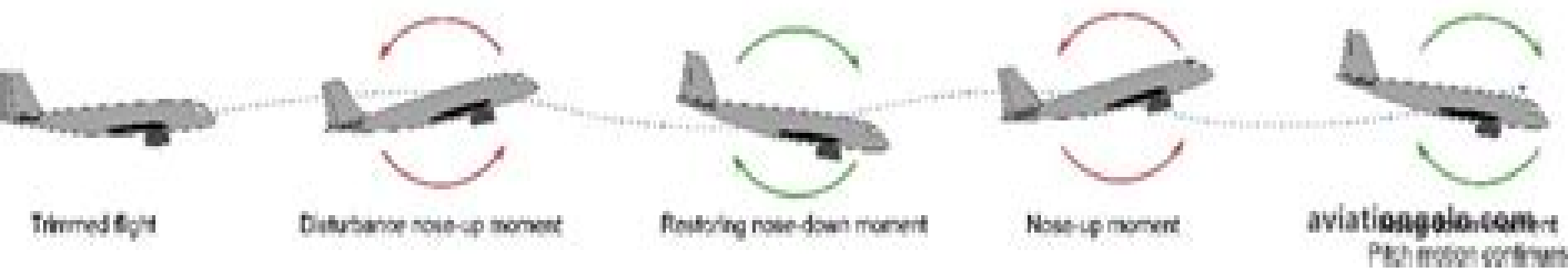
(c) Static stable & dynamically neutral stability
