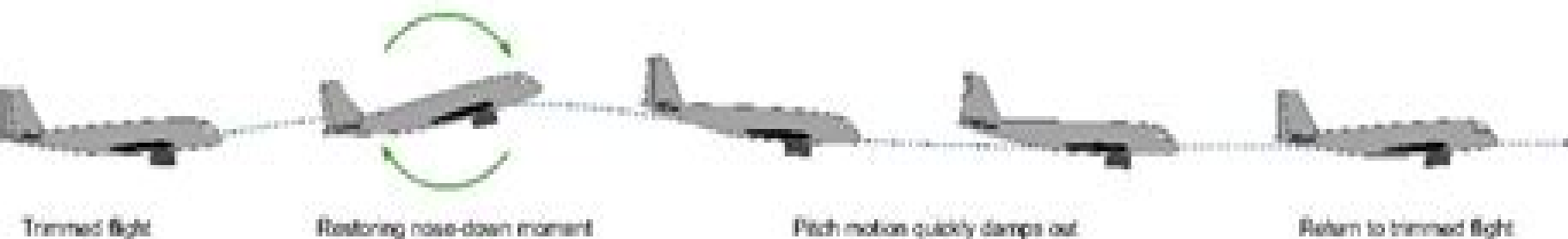
(a) Static & dynamically stable
