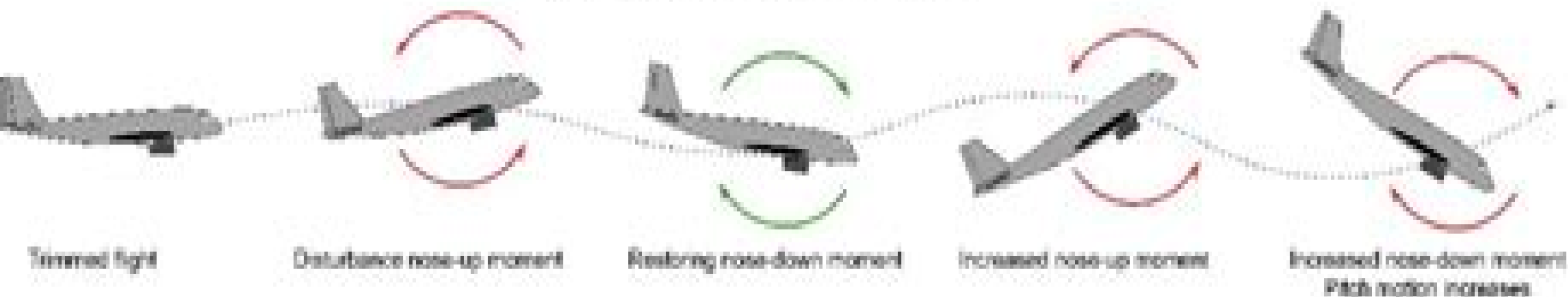
(b) Static stable & dynamically unstable
