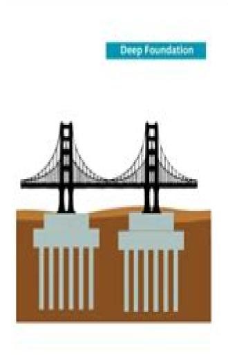
**Definition:** Foundations placed deep underground for heavy structures or weak soil conditions. **Ideal for:** High-rise buildings, bridges, and large industrial projects.
