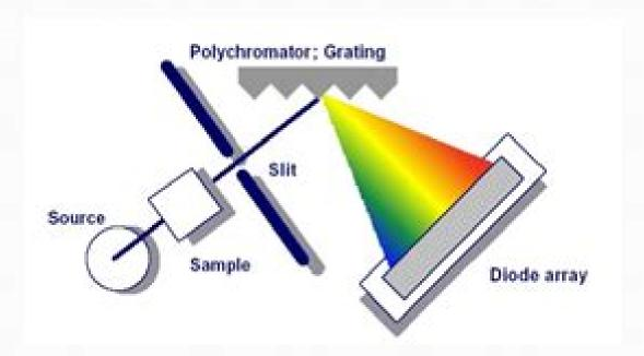
The diode arrays work in parallel simultaneously monitoring all the wavelengths
