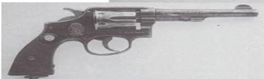
Fig. 63, 64. Smith & Wesson, Military & Police, 38 calibre, s/n 821502. This variation displays the shorter barrel, 38/380 calibre designation on the barrel and the C/Arrow stamp. CWM collection / Kent Photo
