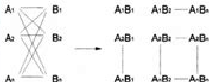
Figure 1.2. (A) In general, in a conventional synthesis one starting material A reacts with one reagent B resulting in one product AB. (B) In a combinatorial synthesis different building blocks of type A (A 1 -A n ) are reacted simultaneously with different building blocks of type B (B 1 -B m ) according to combinatorial principles, i.e. each starting material A i reacts separately with all reagents B resulting in a combinatorial library A 1 -B 1 -B m .
