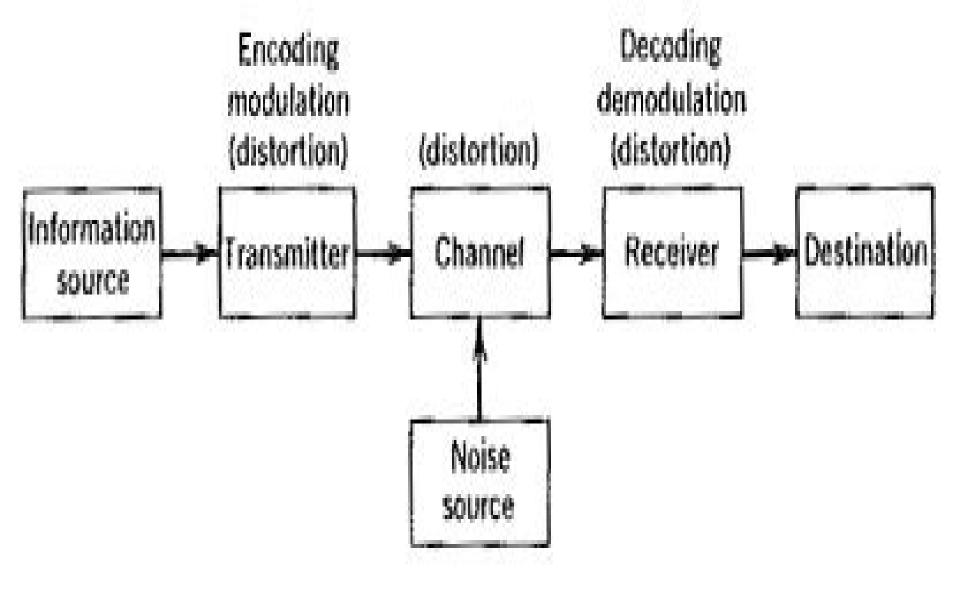
FIGURE 1-1 Block diagram of communications system.
